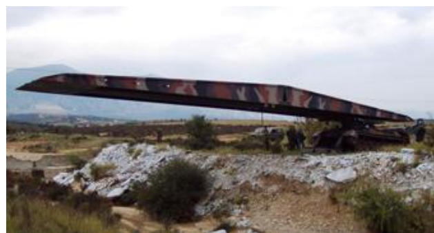
Fig. 1. The deployable bridge built by mutual displacement and sliding of the stacked span blocks
