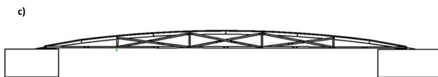
Fig. 25. a) The bridgelayer is ready for deploying the bridge over an obstacle; b) The bridge deployment process; c) The bridge in operational condition
