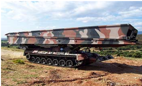
Fig. 1. The deployable bridge built by mutual displacement and sliding of the stacked span blocks
