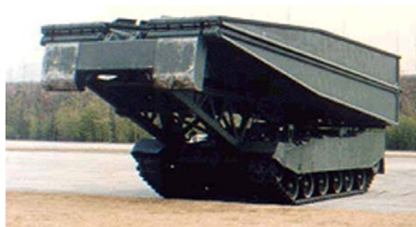
Fig. 2. The stowed bridge transport package disposed on a tank bridgelay and developed in "scissors" like deployment principle
